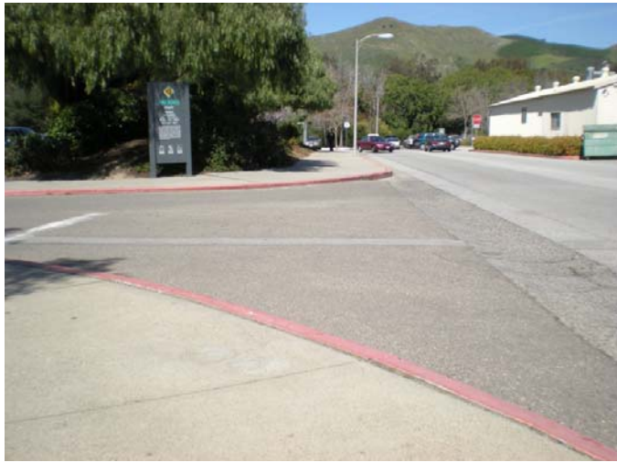
Figure 9.2.C: The Cal Poly transition campus map indicates curb ramps should be at both sidewalks.
