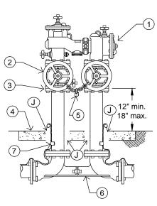
DOUBLE CHECK DETECTOR Use when on-site system includes fire hydrants (4" - 10" only)
