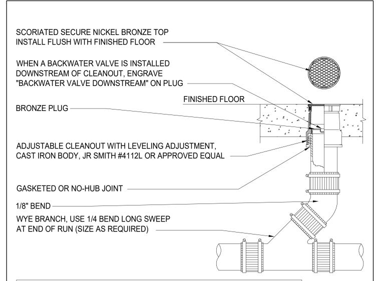
CLEANOUTS IN PIPING 2" OR LESS SHALL HAVE A CLEARANCE OF NOT LESS THAN 18" X 18" IN FRONT OF THE CLEANOUT, CLEANOUTS IN PIPING LARGER THAN 2" INCHES SHALL HAVE A CLEARANCE OF NOT LESS THAN 24" X 24".
